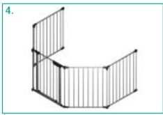
Position HearthGate<sup>™</sup> to desired shape, taking into account recommended 20" minimum distance described in "Important Notes" on page 2. It may be necessary to remove or add section/s to gate to fit your application.
